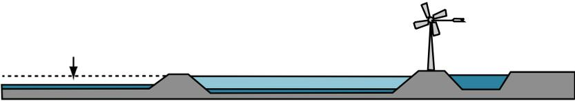
A Bosman mill will empty the retention area onto the "boezem " (main polder channel) until the water reaches the standard level of -1.2 m NAP
